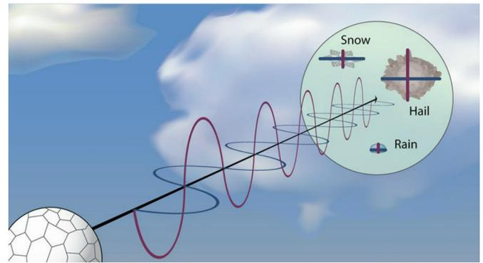
Dual polarization can discern the type of precipitation. Image courtesy: NOAA.
