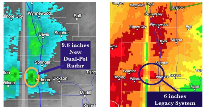
With dual polarization, excessive rainfall can be detected faster so more timely warnings can be issued.
